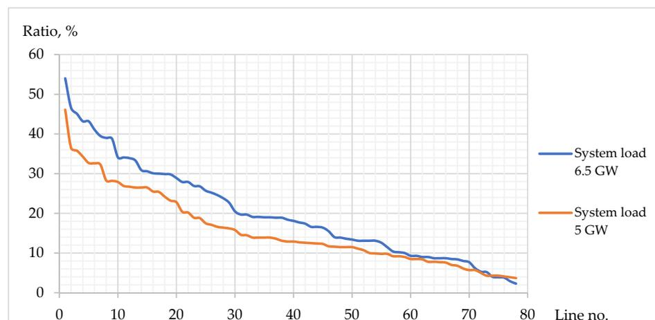
**Figure 7.** Graphs of Ratio vs. number of 330 kV lines with system load of 5 GW and 6.5 GW, respectively.
