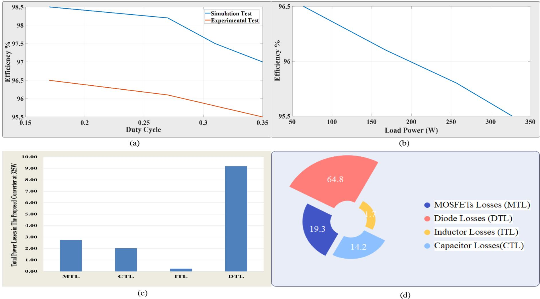
**Figure 14.** Efficiency of the proposed converter (a) vs. duty cycle and (b) vs. load power watts; (c) ( $T_{PLPC}$ ) at 325 W and 500 V output voltage; (d) percentage losses of the elements in the converter at 325 W.
