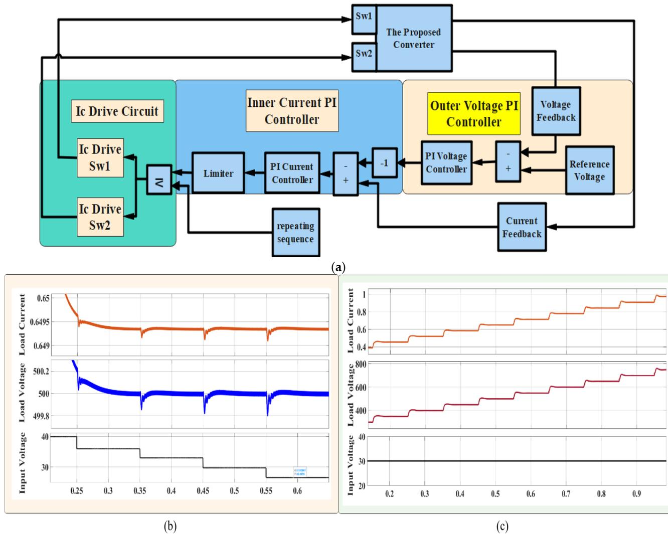
**Figure 7.** (a) Control strategy of the proposed converter; (b) output voltage of the proposed converter at variable input voltage; (c) variable output voltage at fixed input voltage.
