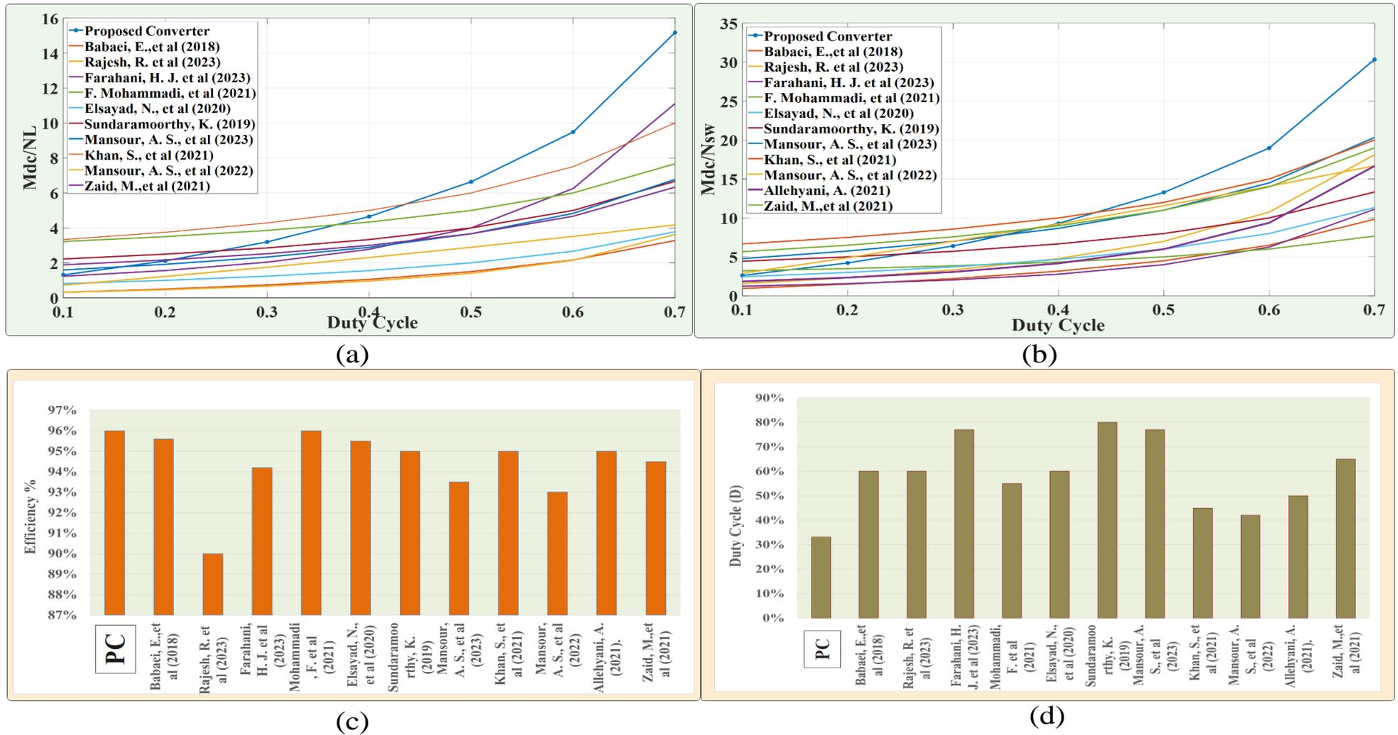
**Figure 6.** (a) Voltage gain  $M_{dc}$ /number of inductors (NL) vs. duty cycle. (b) Voltage gain  $M_{dc}$ /number of switches (NSW) vs. duty cycle. (c) Efficiency comparison of the proposed converter vs. previous work. (d) Duty cycle comparison of the proposed converter vs. previous work, where (PC) is the proposed converter.
