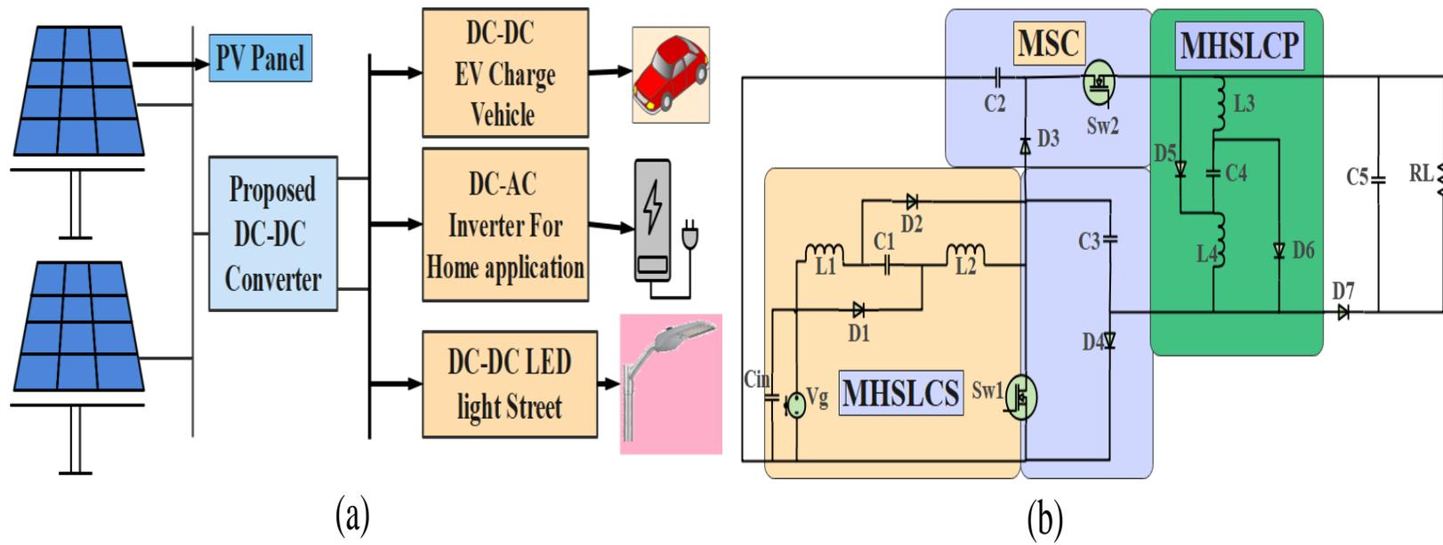
**Figure 1.** (a) The proposed converter integrated with PV Panels with applications. (b) The proposed DC–DC converter.
