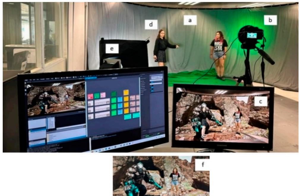
**Figure 3.** Chroma Virtual Production Set tested at the lab. (a) Chroma Backdrop; (b) Camera with tracking system; (c) Reference Monitor; (d) Talent with PCap system; (e) Lights; (f) Realtime Compositing.
