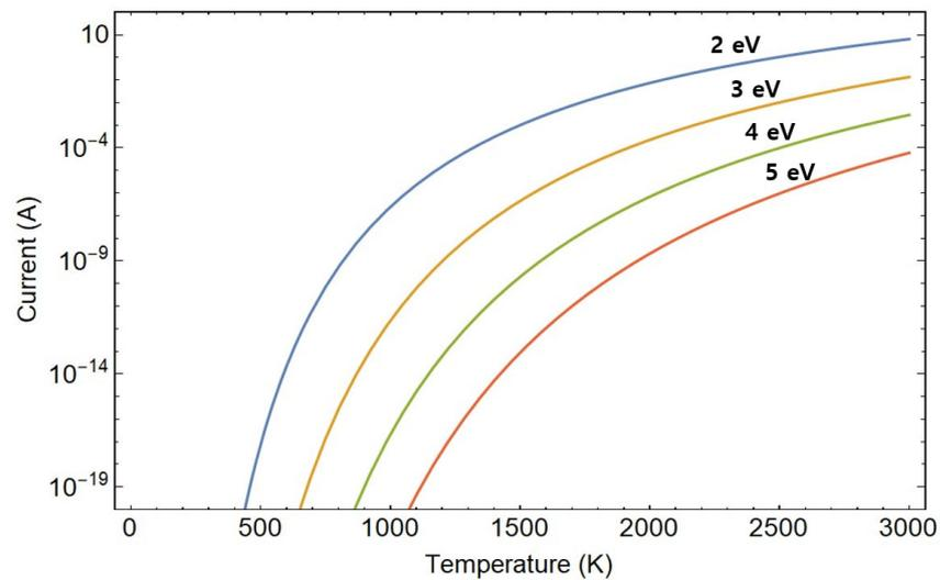
**Figure 3.** One-dimensional current with temperature for various materials characterized by distinct work functions. The electric field is zero, and only thermionic emission is considered. The calculation of the one-dimensional current was conducted for materials with a Fermi energy of 4.57 eV and various work functions, specifically 2, 3, 4, and 5 eV.
