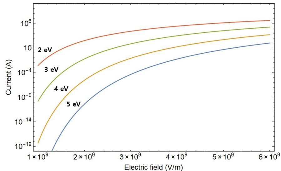
**Figure 4.** One-dimensional current plotted against the accelerating field for materials with varying work functions. The temperature is zero, and only field emission is considered. The calculation involved determining the one-dimensional current for materials with a common Fermi energy of 4.57 eV and different work functions, specifically 2, 3, 4, and 5 eV.
