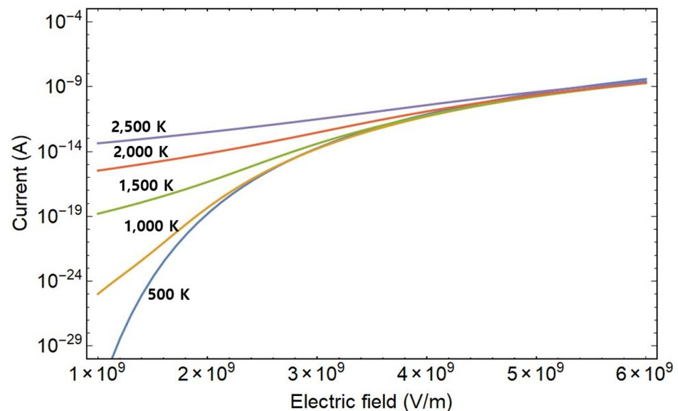
**Figure 5.** One-dimensional current of carbon nanotubes plotted against the accelerating field. In the case of carbon nanotubes, the work function and Fermi level are specified as 4.56 eV and 4.57 eV, respectively. The represented temperatures ascend from bottom to top, representing 500, 1000, 1500, 2000, and 2500 K.
