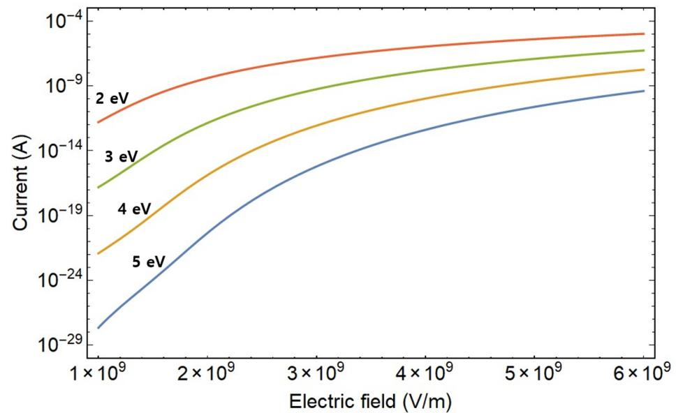
**Figure 6.** One-dimensional current plotted against the applied electric field for materials featuring various work functions, all at a constant temperature of 1000 K. In the sequence from top to bottom, the depicted work functions correspond to 2, 3, 4, and 5 eV.
