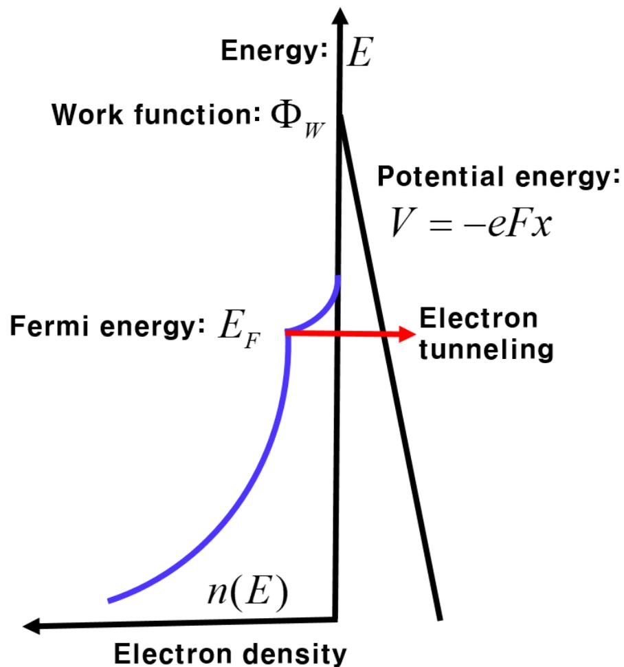
**Figure 1.** Diagram illustrating generalized electron emission in one-dimensional materials. An accelerating field is directed along the  $x$ -axis and applied to the metal. Thermally excited electrons with energy levels surpassing the vacuum threshold engage in thermionic emissions. Electrons experiencing a strong electric field, with energy levels below the vacuum threshold, partake in quantum tunneling, constituting the generalized field emission.
