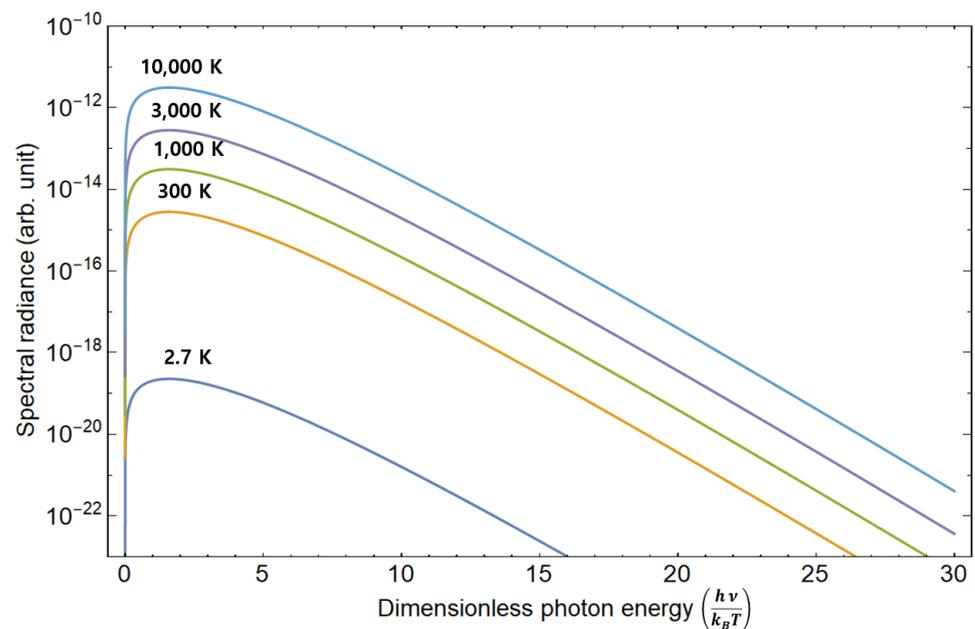
**Figure 2.** Spectral radiance presented as dimensionless photon energy for various temperatures in one-dimensional materials. The spectral radiance, as defined in Equation (9), is represented with dimensionless photon energy ( $\frac{h\nu}{k_B T}$ ) across different temperatures in one-dimensional materials. The sequence of temperatures, from bottom to top, corresponds to 2.7, 300, 1000, 3000, and 10,000 K.
