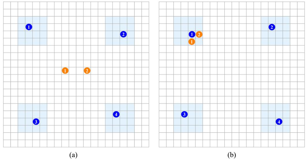
**Figure 3.** Illustration of the pursuit domain environment. (a) The initial state of the environment features two orange predators randomly placed in the central area, and four blue prey randomly placed in the surrounding light blue areas. (b) An illustration of prey capture, depicting both predators simultaneously positioned within the neighboring grid to the prey.
