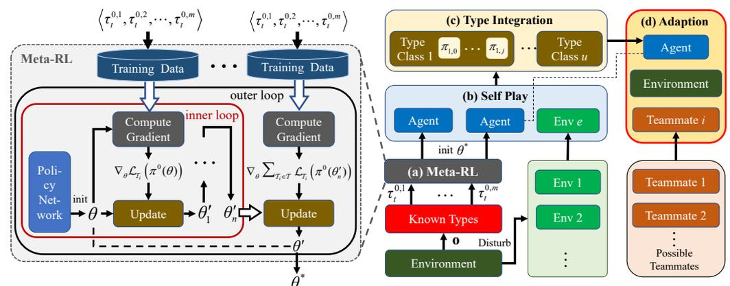
**Figure 1.** The framework diagram of the FEAT algorithm. (a) Acquisition of Meta-RL policy using a small number of teammate types. (b) Self-play generation of a diverse type repository by the Meta-RL policy in a perturbed environment. (c) Calculation of diversity metrics and cluster of the diverse type repository. (d) Online identification and adaptation of teammates during ad hoc agent cooperation.
