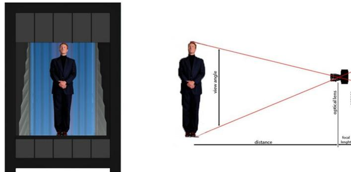
**Figure 3.** Comparison showing the final result of an OLOS<sup>®</sup> installation (**left**) and the parameters that must be taken into account during the recording phase (**right**) to have a suitable result during the visualization.
