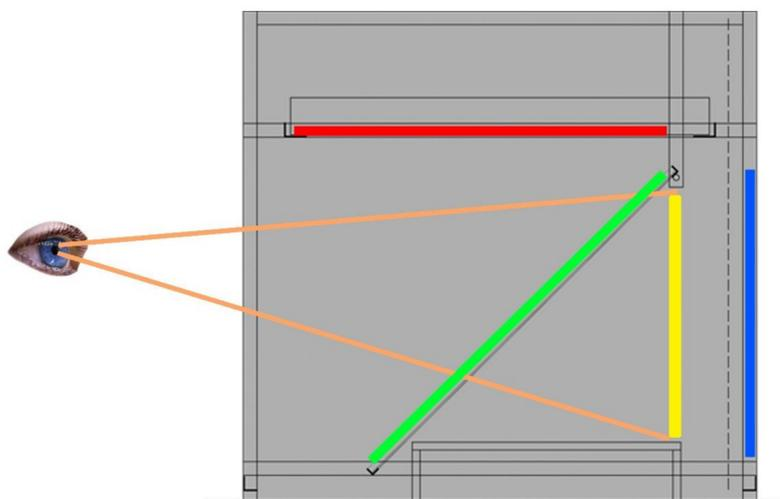
**Figure 1.** This figure shows the reflection (yellow) of an image generated by any type of source (red) by means of a transparent and reflective surface placed (green) at 45° from the ground.
