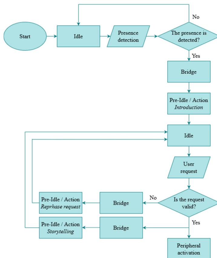
**Figure 2.** Simplified example of a single-scene storytelling flowchart showing the interactions managed within the O<sup>®</sup>EM, in which it is possible to distinguish various states, such as idle, pre-idle, action, and bridge.
