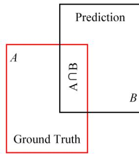
Figure 4. Schematic diagram of the IoU.
