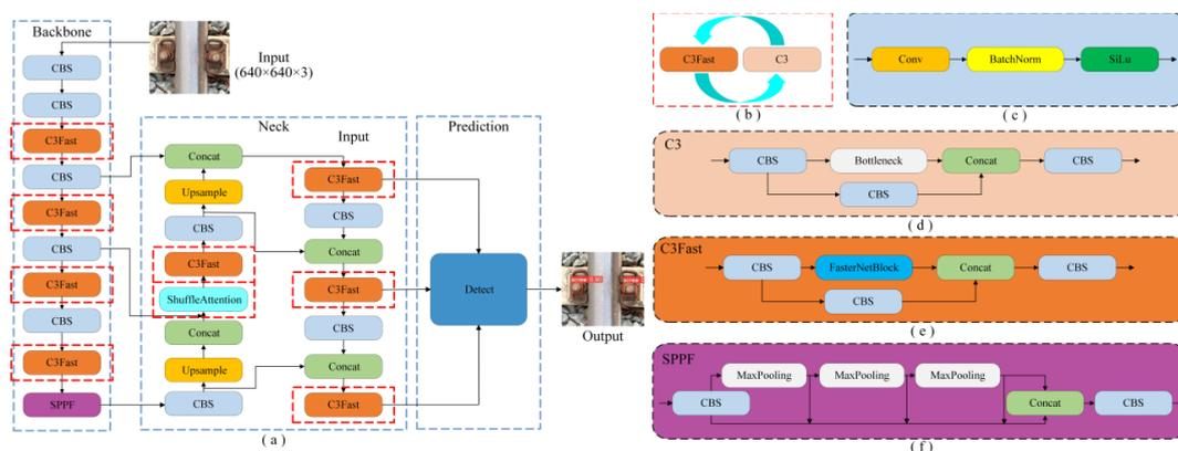
**Figure 2.** Scheme of FSS-YOLO: (a) structure of the proposed model; (b) the light-weight module replacement; (c) CBS module; (d) C3 module; (e) C3Fast module; and (f) SPPF module.
