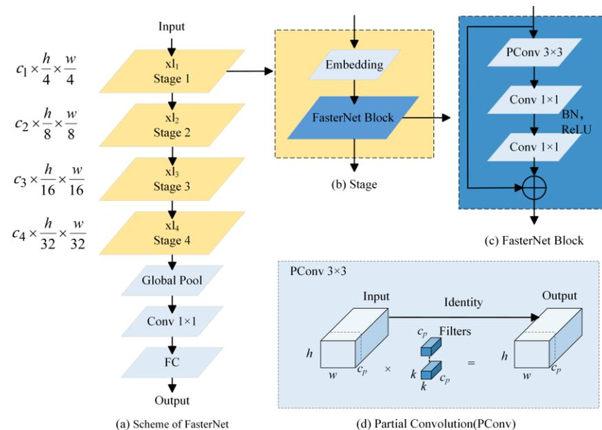
**Figure 3.** Scheme of FasterNet: (a) FasterNet structure; (b) schematic diagram of each stage; (c) schematic diagram of the FasterNet Block; and (d) schematic diagram of the PConv mechanism.
