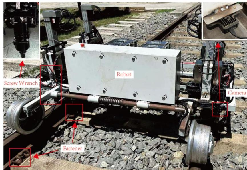
**Figure 1.** Fastener screw maintenance robot: The small picture in the upper left corner is the electric screw wrench, which is adapted for disassembling and assembling the fastener screws. The small picture in the upper right corner is the depth camera, which is used for the detection and location of fastener screws.
