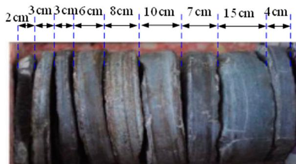
**Figure 4.** Core discing phenomenon in the borehole 2 of the roadway sidewall.
