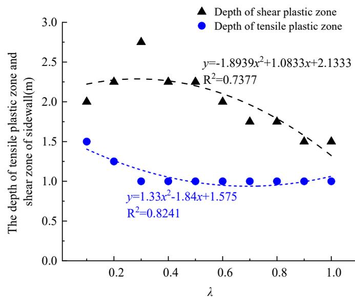
**Figure 14.** Scatter of the relationship between the  $\lambda$  and the depth of tensile plastic zone and shear zone of the roadway sidewall.
