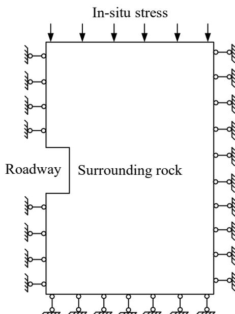
Figure 6. Boundary conditions used in rock mass.
