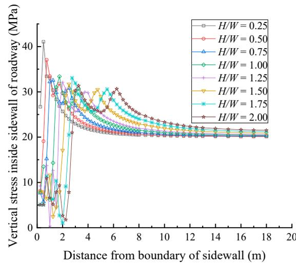
Figure 11. Vertical stress monitoring curves inside the sidewall of the roadway under different  $h/w$ .
