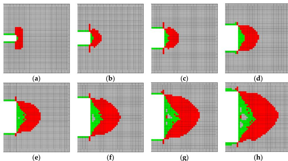
**Figure 7.** Distribution of tensile and shear plastic zones in roadway sidewall under various height-width ratio  $h/w$  (green is tensile and red is shear): (a)  $h/w = 0.25$ ; (b)  $h/w = 0.50$ ; (c)  $h/w = 0.75$ ; (d)  $h/w = 1.00$ ; (e)  $h/w = 1.25$ ; (f)  $h/w = 1.50$ ; (g)  $h/w = 1.75$ ; (h)  $h/w = 2.00$ .
