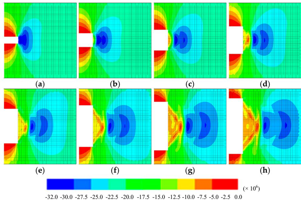
**Figure 10.** Vertical stress of sidewall under various height-width ratio  $h/w$  (green is tensile and red is shear): (a)  $h/w = 0.25$ ; (b)  $h/w = 0.50$ ; (c)  $h/w = 0.75$ ; (d)  $h/w = 1.00$ ; (e)  $h/w = 1.25$ ; (f)  $h/w = 1.50$ ; (g)  $h/w = 1.75$ ; (h)  $h/w = 2.00$ .
