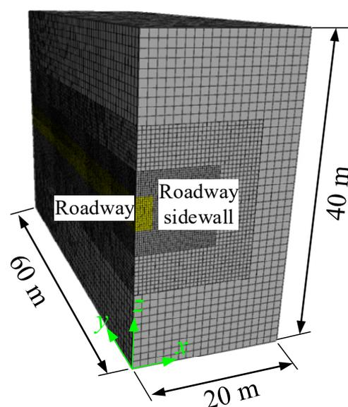
**Figure 5.** Three-dimensional model used for numerical calculation of roadway sidewall failure (height-width ratio  $h/w = 1$ ).
