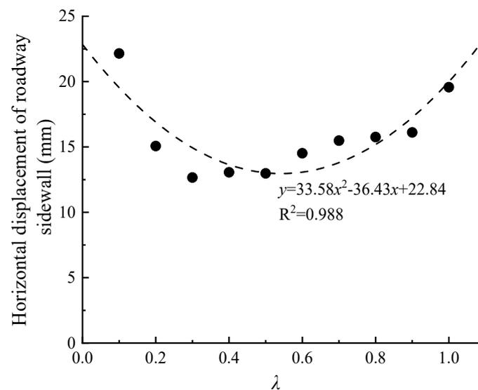
**Figure 15.** Relationship between  $\lambda$  and horizontal displacement of the roadway sidewall.
