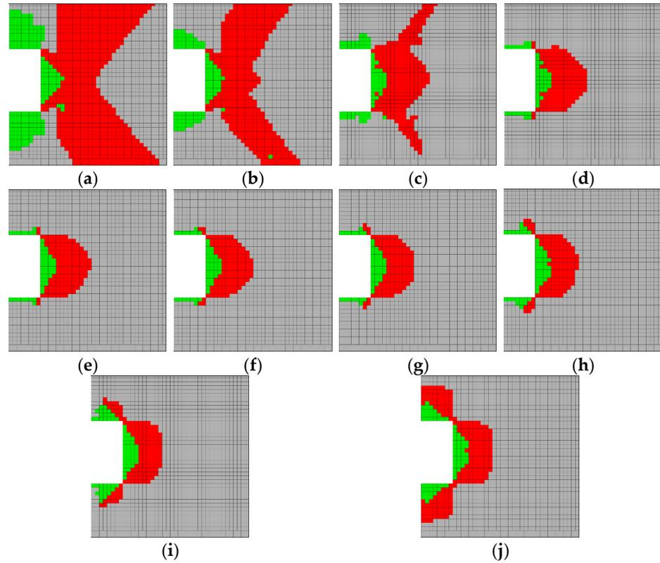
**Figure 13.** Distribution of tensile and shear plastic zones in the roadway sidewall under different lateral pressure coefficients  $\lambda$  (green is tensile and red is shear): (a)  $\lambda = 0.1$ ; (b)  $\lambda = 0.2$ ; (c)  $\lambda = 0.3$ ; (d)  $\lambda = 0.4$ ; (e)  $\lambda = 0.5$ ; (f)  $\lambda = 0.6$ ; (g)  $\lambda = 0.7$ ; (h)  $\lambda = 0.8$ ; (i)  $\lambda = 0.9$ ; (j)  $\lambda = 1.0$ .
