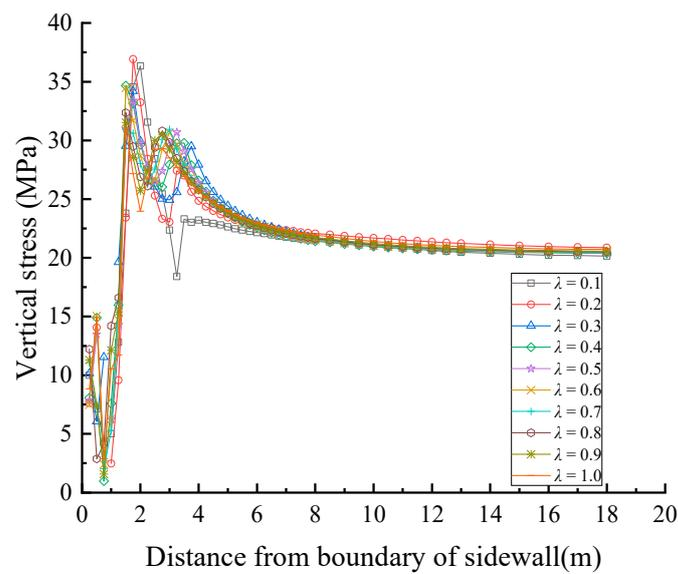
**Figure 17.** Vertical stress monitoring curves inside the sidewall of the roadway under different  $\lambda$ .
