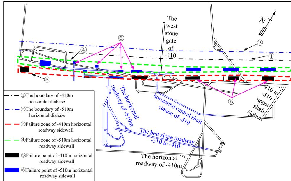
**Figure 1.** Distribution of roadway failure occurrence at the levels  $-410$  m and  $-510$  m in Datai coal mine.
