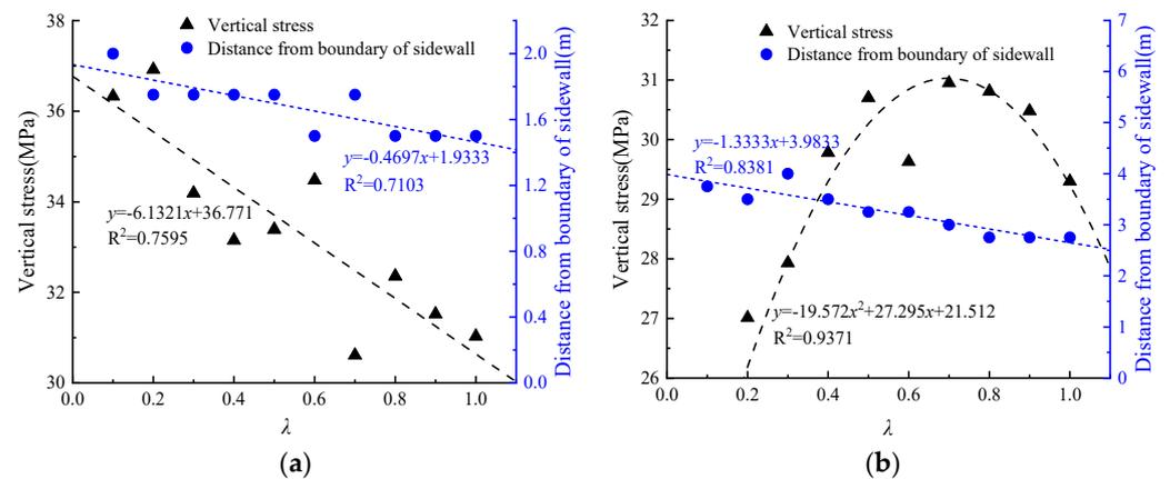
**Figure 18.** Relationship between  $\lambda$  and maximum vertical stress inside of the roadway sidewall: (a) First stress peak point inside of roadway sidewall; (b) Second stress peak point inside of sidewall.
