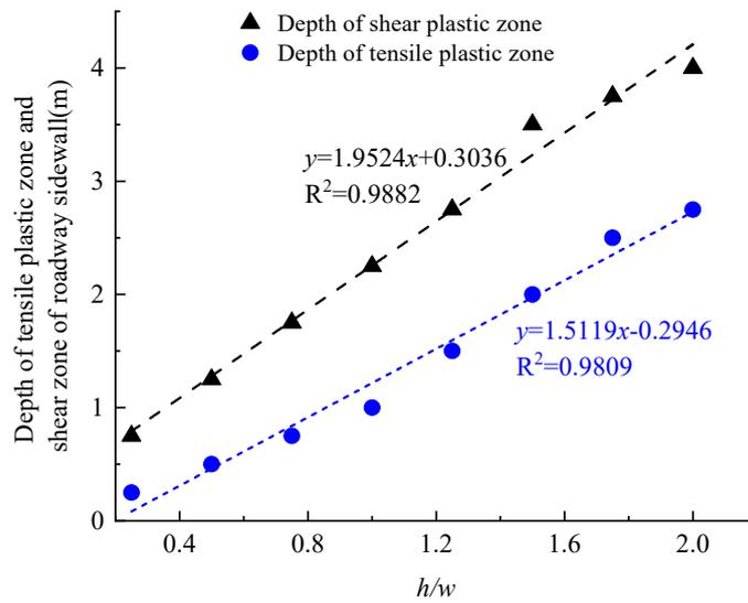
**Figure 8.** Scatter of the relationship between  $h/w$  and the depth of the tensile plastic zone and shear plastic zone of a roadway sidewall.
