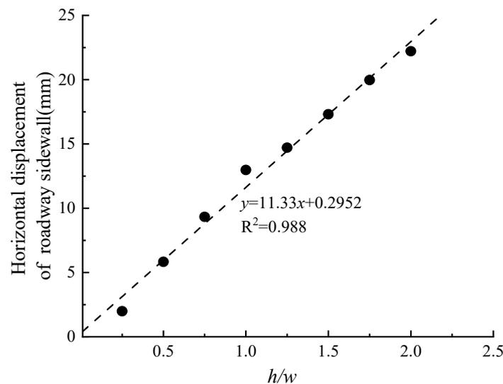
**Figure 9.** Relationship between  $h/w$  and horizontal displacement of the roadway sidewall.
