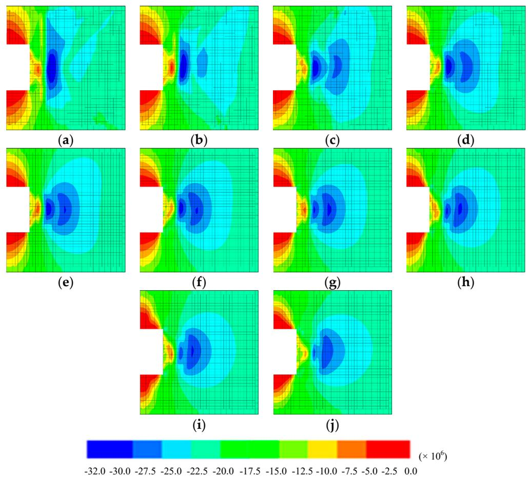
**Figure 16.** Vertical stress distribution in the roadway sidewall under different lateral pressure coefficient  $\lambda$  (green is tensile and red is shear): (a)  $\lambda = 0.1$ ; (b)  $\lambda = 0.2$ ; (c)  $\lambda = 0.3$ ; (d)  $\lambda = 0.4$ ; (e)  $\lambda = 0.5$ ; (f)  $\lambda = 0.6$ ; (g)  $\lambda = 0.7$ ; (h)  $\lambda = 0.8$ ; (i)  $\lambda = 0.9$ ; (j)  $\lambda = 1.0$ .
