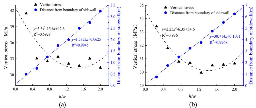
Figure 12. Relationship between  $h/w$  and maximum vertical stress inside of the roadway sidewall: (a) First stress peak point inside of roadway sidewall; (b) Second stress peak point inside of roadway sidewall.
