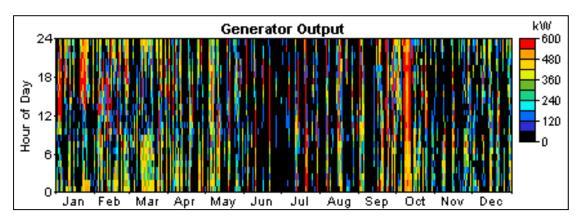
Figure 11. 600 kW diesel generator use in wind/diesel system without VRB storage.
