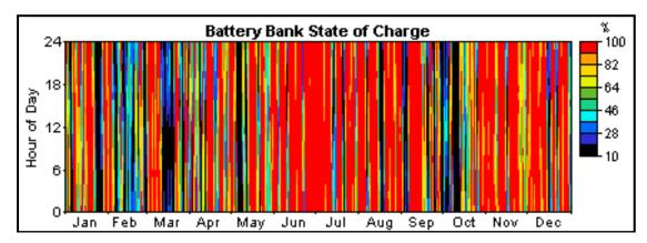
Figure 8. Vanadium Redox Battery (VRB) state of charge variations over a twelve month period.
