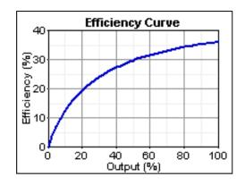
The efficiency curve above demonstrates two aspects of diesel power generation. Firstly, in general, efficiency is very low. Operating at a peak of around 35% efficiency, most of the energy supplied to a diesel generator is wasted. Secondly, there is a marked reduction in efficiency with a reduction in power output. For this reason, a constraint is placed on the system within HOMER to limit the minimal power output of the diesel generators to 30% of their overall capacity.
