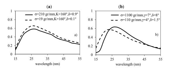
Figure 4. Efficiency curve of the gratings with the parameters listed in Table 1: (a) CDM; (b) OPM.
