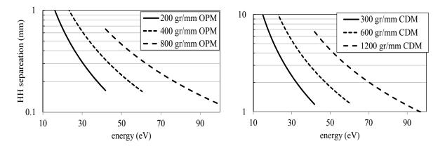
Figure 9. Separation between neighboring harmonics at the monochromator exit slit.
