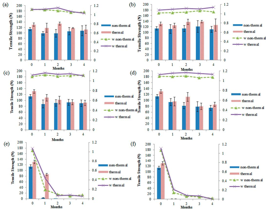
**Figure 8.** Tensile strength and weight along the CD of recycled Kevlar<sup>®</sup>/PET/LPET nonwoven geotextiles of (a) H<sub>2</sub>O/23 °C, (b) H<sub>2</sub>O/50 °C, (c) CH<sub>3</sub>COOH/23 °C, (d) CH<sub>3</sub>COOH/50 °C, (e) NaOH/23 °C, and (f) NaOH/50 °C, as related to the implementation of thermal treatment.
