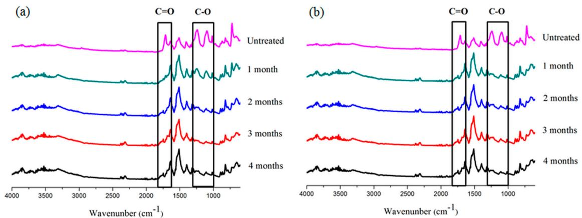
**Figure 7.** FT-IR spectra of nonwoven geotextiles that are immersed in NaOH at (a) 23 °C and (b) 50 °C.
