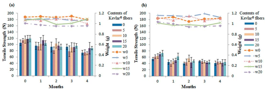
**Figure 4.** Tensile strength and weight along the (a) CD and (b) MD of recycled Kevlar®/PET/LPET nonwoven geotextiles that are immersed in CH<sub>3</sub>COOH at 50 °C for 4 months.
