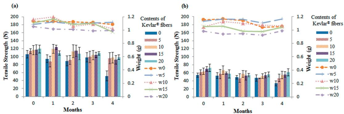
**Figure 3.** Tensile strength and weight along the (a) CD and (b) MD of recycled Kevlar®/PET/LPET nonwoven geotextiles that are immersed in CH<sub>3</sub>COOH at 23 °C for 4 months.
