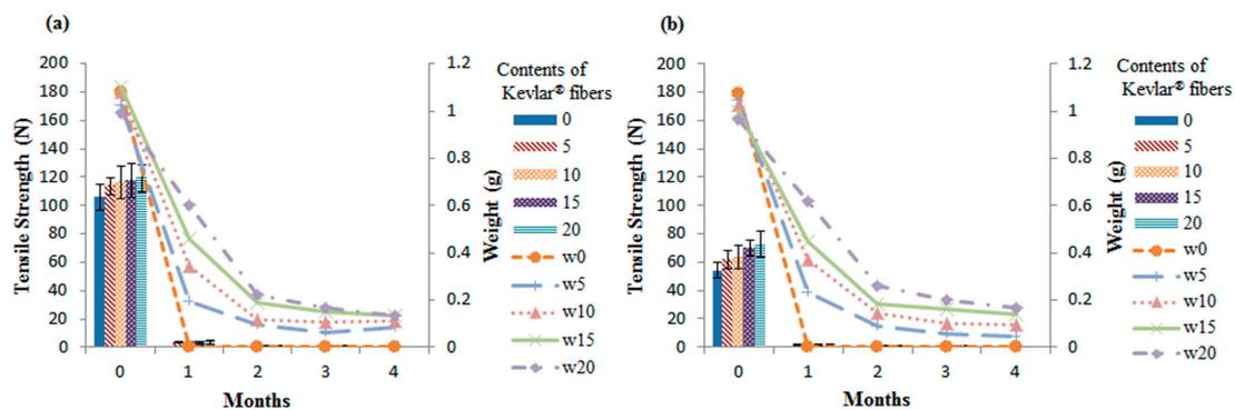
**Figure 5.** Tensile strength and weight along the (a) CD and (b) MD of recycled Kevlar®/PET/LPET nonwoven geotextiles that are immersed in NaOH at 23 °C for 4 months.
