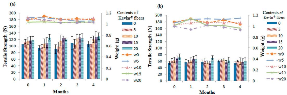
**Figure 1.** Tensile strength and weight along the (a) cross machine direction (CD) and (b) machine direction (MD) of recycled Kevlar®/PET/LPET nonwoven geotextiles that are immersed in H<sub>2</sub>O at 23 °C for 4 months.
