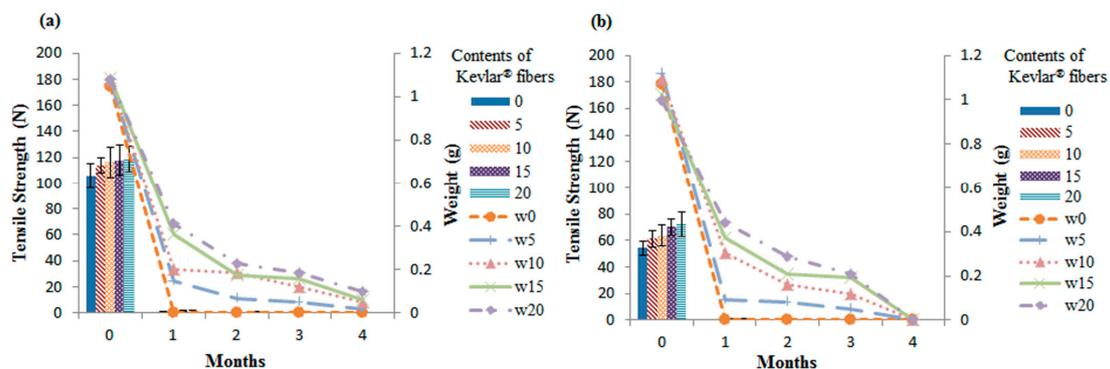
**Figure 6.** Tensile strength and weight along the (a) CD and (b) MD of recycled Kevlar®/PET/LPET nonwoven geotextiles that are immersed in NaOH at 50 °C for 4 months.
