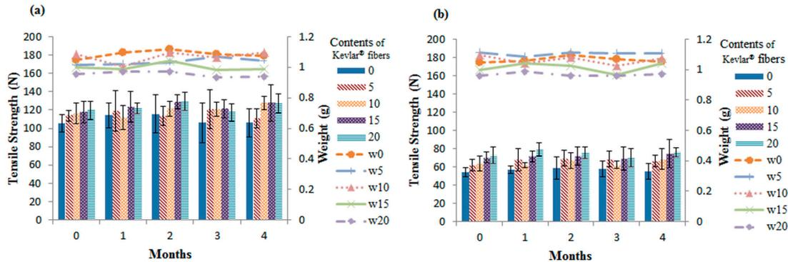
**Figure 2.** Tensile strength and weight along the (a) CD and (b) MD of recycled Kevlar®/PET/LPET nonwoven geotextiles that are immersed in H<sub>2</sub>O at 50 °C for 4 months.
