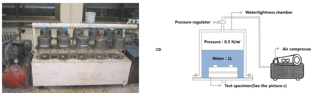
Figure 10. Permeability test chamber (output).
