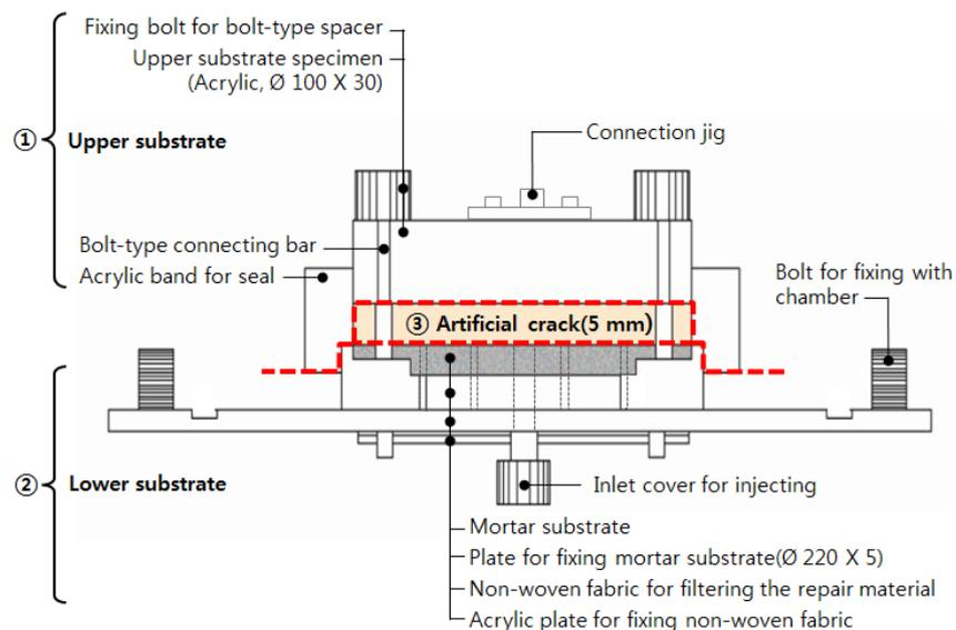
Figure 2. Artificial crack specimen structure concept.
