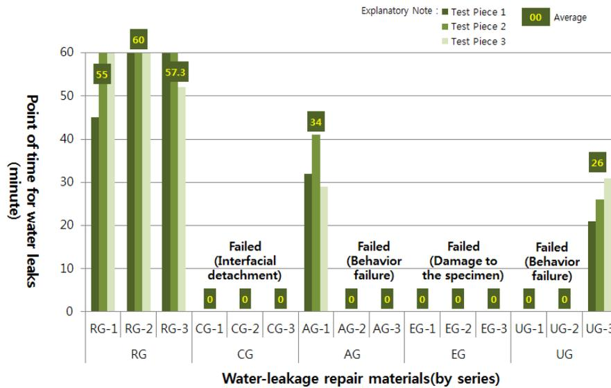
Figure 12. Leakage repair material (by series) water leakage response time.
