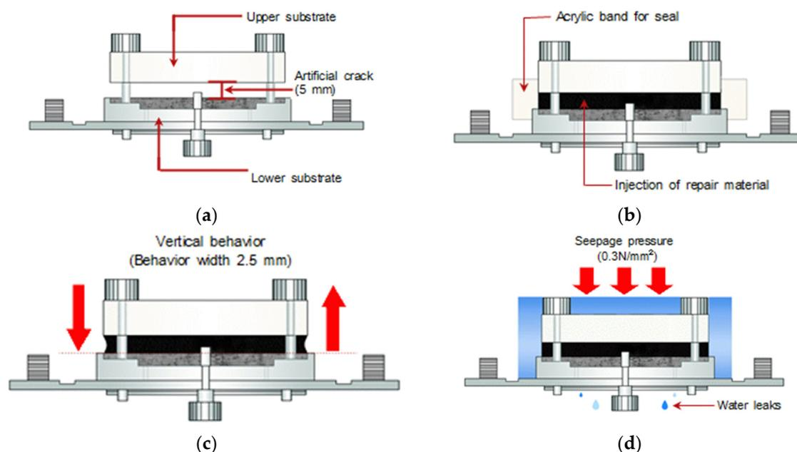
**Figure 1.** Overview of the artificial-crack-behavior test. (a) 5-mm-artificial-crack test specimens; (b) Injection of repair material; (c) Vertical crack behavior (100 cycles); (d) Water pressure (60 mins).
