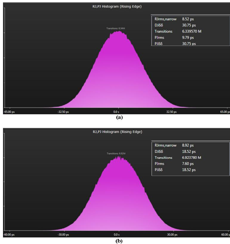
Figure 9. Jitter Histogram of CLKA and CLKB. (a) Jitter of CLKA; (b) Jitter of CLKB.
