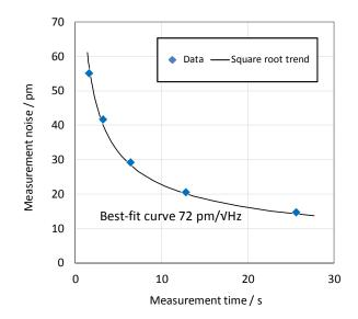
**Figure 2.** Experimental demonstration of the reduction of measurement noise as a function of data acquisition time for the ZYGO Nexview<sup>TM</sup> 3D interference microscope.
