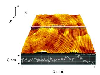
**Figure 1.** An example of optical surface topography measurement requiring nm-level sensitivity to surface heights.
