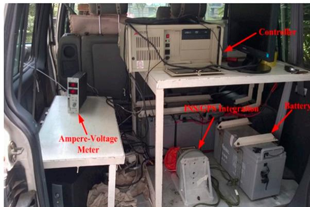
Figure 12. The vehicle loaded navigation equipment.
