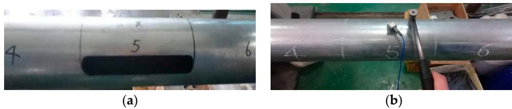
Figure 18. Actual damage and measured response. (a) Damage hole; (b) Hammer excitation.
