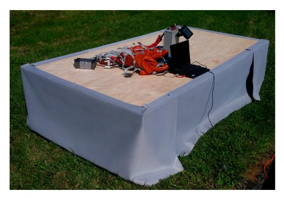
**Figure 1.** Shroud with camera. Orange backpack is tethered to the camera and is used to house electronics when the camera system is used in a portable mode.
