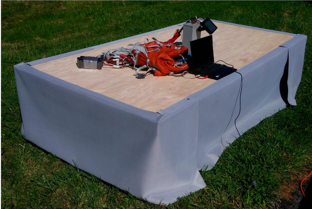
**Figure 1.** Shroud with camera. Orange backpack is tethered to the camera and is used to house electronics when the camera system is used in a portable mode.
