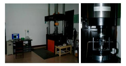
Figure 6. Rock mechanics servo-controlled testing system (Instron 1346).
