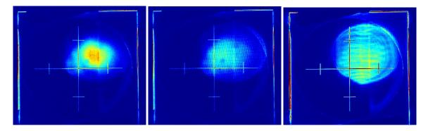
**Figure 5.** Photon spotsize for 50 (**left**), 85 (**middle**) and 150 nm (**right**) wavelength, 15 m downstream of the undulator with automatic optics adjustment in the undulator switched on. Without adjustment, the undulators cannot be closed to produce wavelengths longer than 85 nm because of beam loss.
