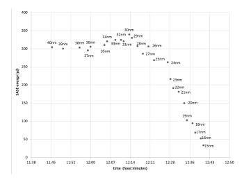
**Figure 3.** Fast wavelength scan at FLASH2 performed while FLASH1 delivered the beam to users at 13.5 nm (electron beam energy 699 MeV). This scan was performed with standard undulator optics (see below).
