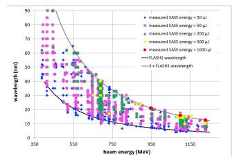
**Figure 2.** Wavelength tunability of FLASH2 for specific electron beam energies. The different symbols and colors refer to the achieved photon pulse energies. The upper and lower limits are given by three times the FLASH1 wavelength as a maximum (for a closed undulator gap) and the FLASH1 wavelength as a minimum.
