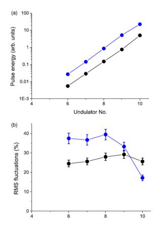
**Figure 7.** Growth of pulse energy (**a**) and fluctuations (**b**) along the undulator for SASE (black) and HLSS (blue). In the HLSS experiment the first four undulators were set to 33 nm and the next six undulators to 11 nm, while in the SASE case all ten undulators modules were set to 11 nm.
