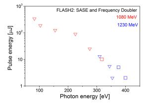
**Figure 10.** Setting the first part of the undulator to twice the final wavelength (squares), the final wavelength that can be reached with reasonable pulse energy is much shorter and has more stable intensity than with setting all undulators to the same resonant wavelength (triangles).
