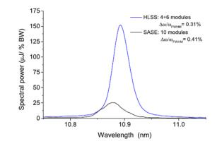
Figure 8. Spectral bandwidth for SASE and HLSS in the same experiment.
