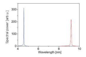
**Figure 11.** Radiation spectra generated in a frequency doubler experiment at FLASH2 tuned to equal pulse energies for the two wavelength taken with a grating spectrometer [14] in the experimental hall. In blue, the spectral line for the second harmonic at 4.5 nm, and in red, the first harmonic at 9 nm are shown. The electron beam energy in this experiment was 1080 MeV and the bunch charge 300 pC.
