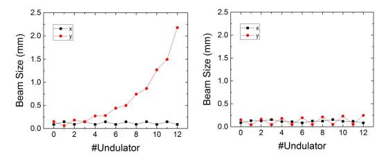
**Figure 4.** Simulated beam size (in mm) along the undulator without automatic adjustment (left) and including adjusted focusing to compensate for the additional undulator focusing (**right**) for a beam energy of 380 MeV and an undulator  $K_{rms} = 2$ .
