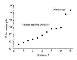
**Figure 12.** The figure shows the photon pulse energy measured after the respective undulator in FLASH2. Undulators 1 to 10 were set to reverse tapering while the final two act as an afterburner, leading to an increase in pulse energy by a factor of 200.
