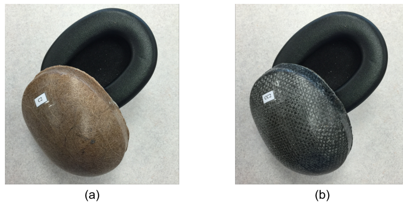
Figure 1. Closed-up view of the composite ear cups assembled with the inner foam lining and cushion: (a) coir fibre-reinforced polypropylene (Coir-PP); and (b) coir/carbon fibre-reinforced polypropylene (Coir/C-PP).
