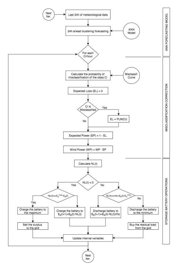
**Figure 2.** Monte Carlo simulation workflow: The simulation is divided into three stages: (1) power output forecast using artificial neural network (ANN); (2) misclassification correction; and, (3) battery storage operations.
