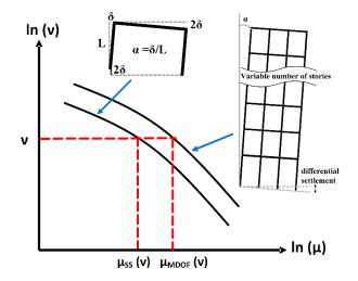
Figure 10. Schematic representation related to the estimation of the ductility transformation factors (DTF).
