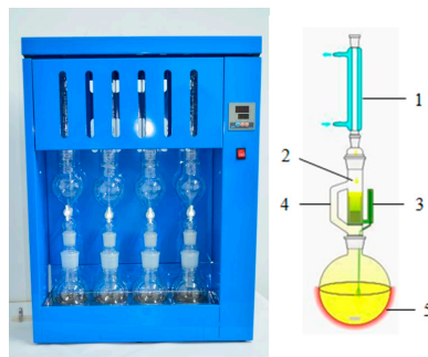
Figure 1. Soxhlet Extractor. Note: 1: condenser tube; 2: extraction tube; 3: siphon tube; 4: connection tube; 5: extraction flask.
