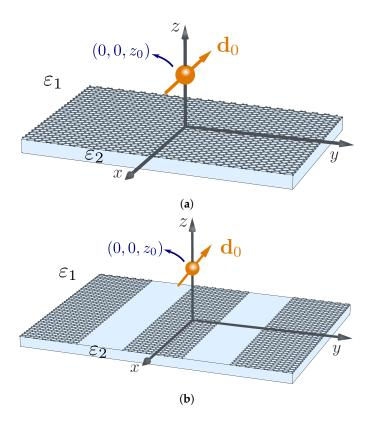
**Figure 1.** The two systems considered in this paper: a graphene sheet (**a**) and a graphene grid of ribbons (**b**) located in between two dielectrics. A nanoparticle is located at position  $\mathbf{r}_0 = (0,0,z_0)$  and is characterized by a polarizability tensor  $\alpha_0$  in vacuum. In addition, a plane wave impinges on the nanoparticle and on graphene coming from  $z = +\infty$ .
