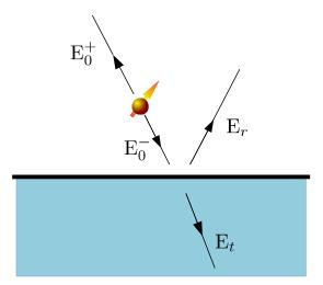
**Figure 2.** Representation of the primary field  $(E_0^{\pm})$ , emitted by a point dipole (represented by the golden ball with an arrow), and the reflected  $(E_r)$  and the transmitted  $(E_t)$  field due to the presence of the interface at z = 0. The  $\pm$  sign in  $E_0^{\pm}$  indicates whether the field is emitted along the positive/negative z direction.
