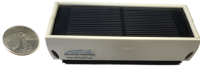
Figure 1. Cellular Track Technologies (CTT)-1000a Internet of things (IoT) wildlife behavior monitoring device.
