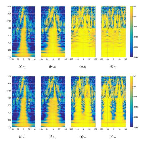
**Figure 11.** Horizontal cross-section through measured frequency-dependent beampatterns of the IKO normalized by the half-octave smoothed magnitude of the loudest direction in  $A_1^* = C_1$ . Decibel values are color coded over frequency in Hertz and azimuth angle in degree.
