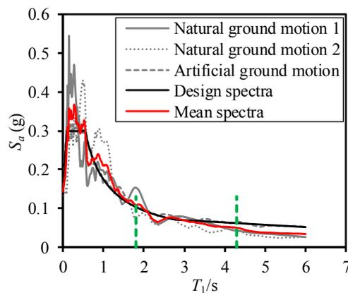
Figure 15. Response spectra of the selected ground motions.
