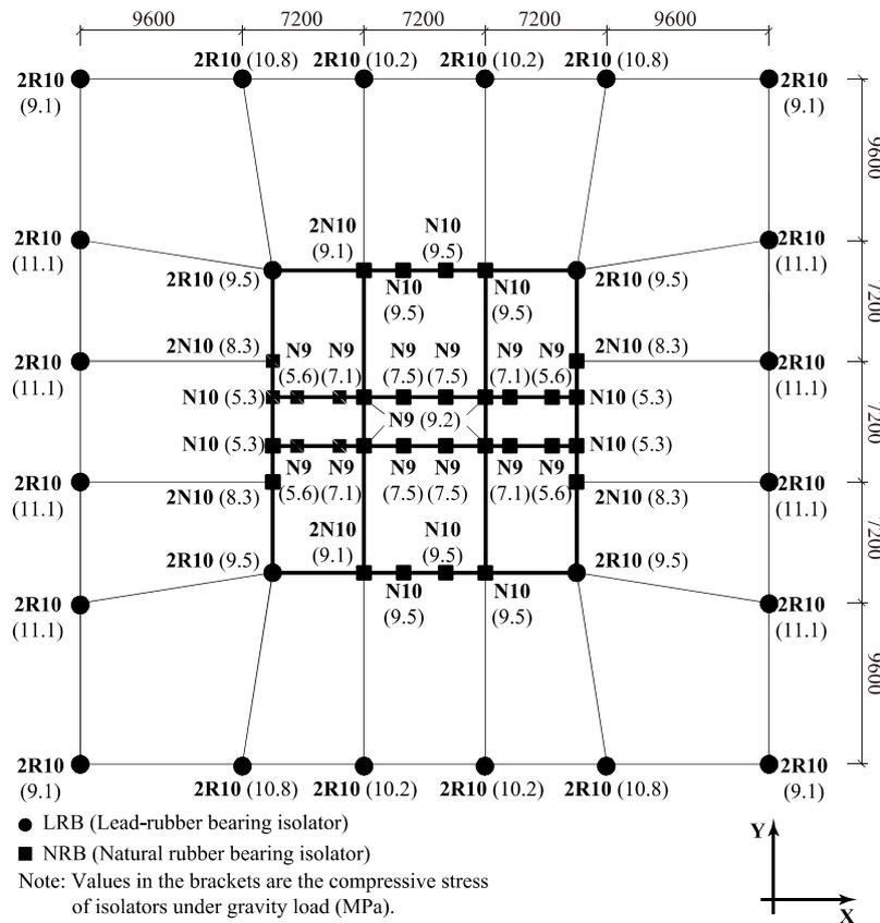
Figure 14. Compressive stress of isolators under gravity load.
