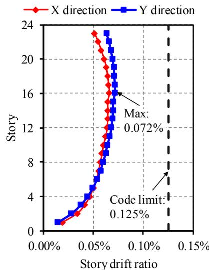
Figure 13. Distribution of inter-story drift ratio of superstructure.
