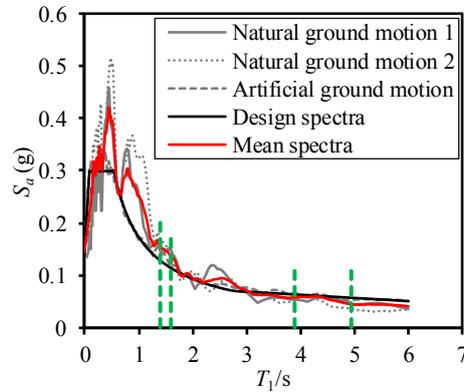
Figure 3. Response spectra of design ground motions.
