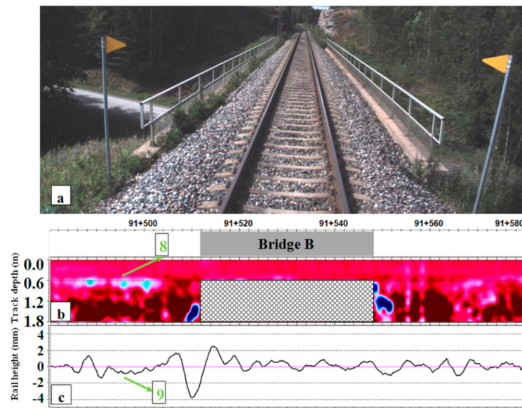
Figure 9. Measurement results of Transition Zone B: (a) photograph of the track; (b) the moisture profile; and, (c) the longitudinal track level.
