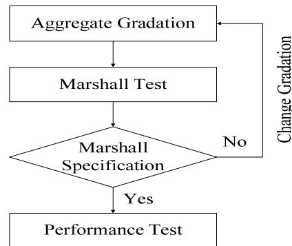
**Figure 1.** Flow chart of stone matrix asphalt (SMA) mixture design.**Table 6.** Results of SMA mixture design.
