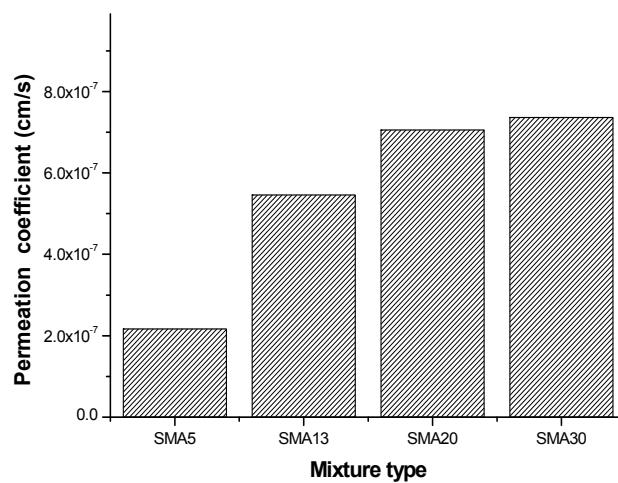
**Figure 3.** Mixture types and permeability coefficients.
