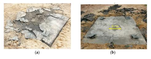
**Figure 11.** Damage of the multi-layer pavement after blast loading: (**a**) damage pattern of the AC layer in field blast test; (**b**) damage pattern of the HSC layer in field blast test.
