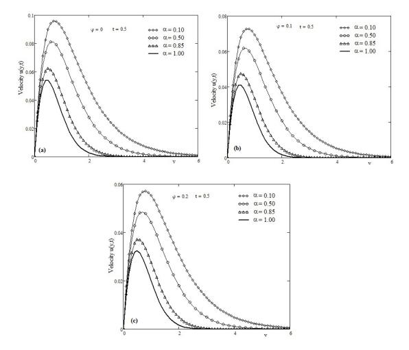
**Figure 3.** Variation of the velocity u(y,t) with the fractional parameter  $\alpha$  and the nanoparticle volume fraction  $\varphi$ . (a) for  $\varphi = 0$ ; (b)  $\varphi = 0.1$ ; (c) for  $\varphi = 0.2$ .
