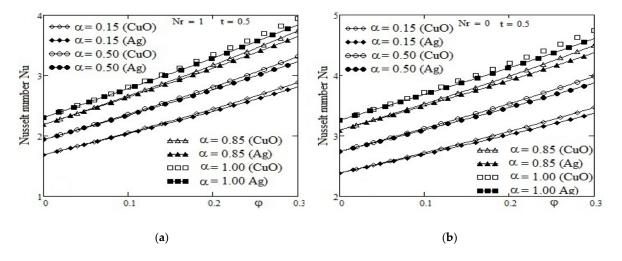
**Figure 2.** Values of the Nusselt number against the nanoparticle volume fraction  $\varphi$  for the two water-based nanofluids. (a) for Nr = 1; (b) for Nr = 0.
