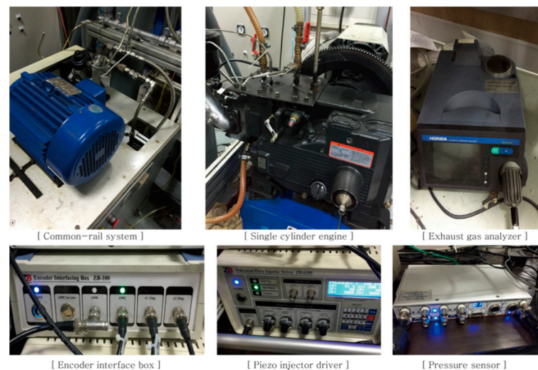
Figure 6. Experiment system of single-cylinder diesel engine.
