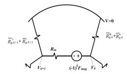
Figure 5. Magnetic circuit of one section in the rotor of SP-PMVM.
