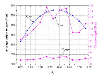
Figure 6. Average torque, cogging torque, and torque ripple of SP-PMVM at different k<sub>st</sub>.
