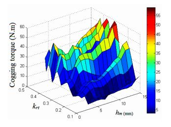
**Figure 9.** Cogging torque at different  $k_{rt}$  and  $h_m$ .
