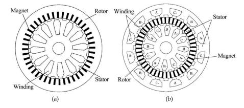
Figure 3. Comparison of the two machines: (a) conventional PMVM; and (b) SP-PMVM.
