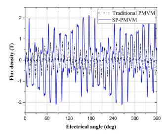
Figure 12. Air gap flux density.
