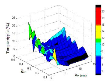
**Figure 10.** Torque ripple at different  $k_{rt}$  and  $h_m$ .
