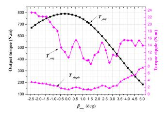
**Figure 7.** Average torque, cogging torque, and torque ripple at different  $\beta_{mec}$ .
