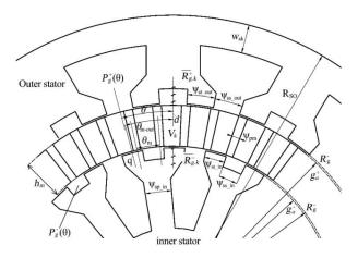
Figure 4. Definition of parameters of SP-PMVM.
