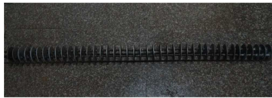
Figure 1. U type tube and fin profile.
