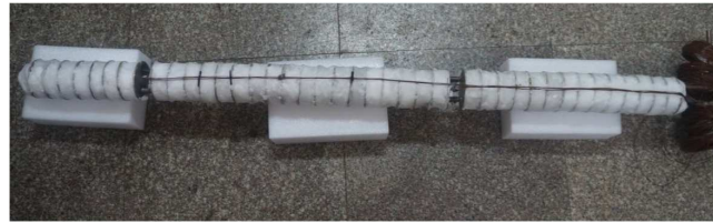
Figure 3. U-tube prefilled with paraffin.
