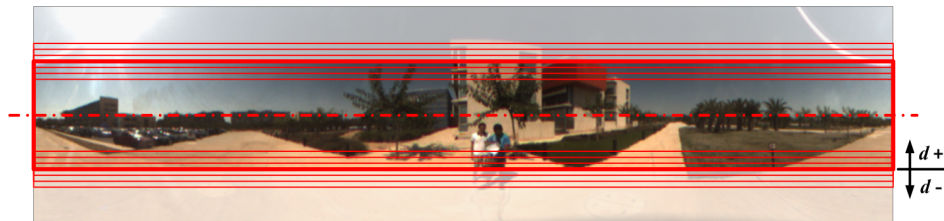
Figure 4. Set of cells defined in a reference panoramic image for height estimation using the central cell correlation technique.
