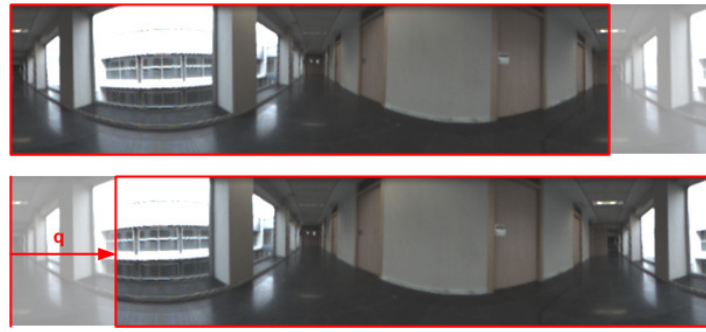
Figure 3. Two panoramic images captured indoors from the same (x, y) position in the floor plane and a change of orientation \phi = 68 deg. The result is a circular shift of the columns.
