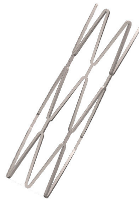
Figure 1. Initial cylindrical configuration of spherical occlusion device.
