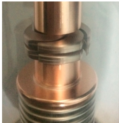
Figure 7. Vacuum interrupter with spiral-type TMF contacts.
