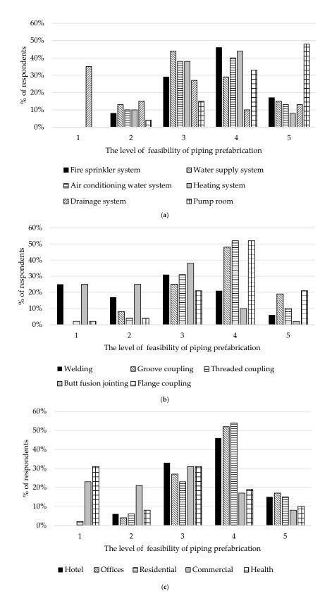
**Figure 4.** Level of feasibility of piping prefabrication. (**a**) the level of feasibility of prefabrication in different types of piping systems; (**b**) the level of feasibility of prefabrication in different connection modes of piping; (**c**) the level of feasibility of prefabrication in different types of projects.
