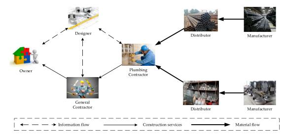
Figure 1. Supply chain of piping construction.
