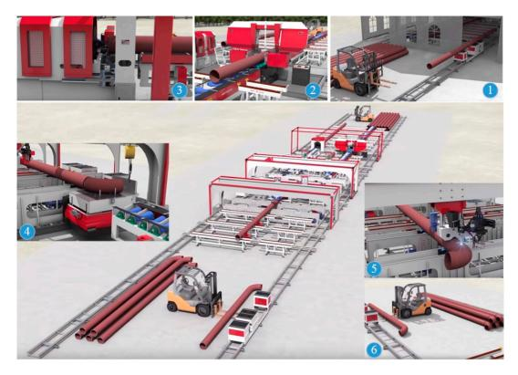
**Figure 9.** Configuration of a pipe fabrication production line. (1) the arrival of standard pipes; (2) high-speed pipe cutting machine; (3) the beveling machine; (4) the piping prefabrication fast fitting-up machine; (5) piping automatic welding machine; (6) the prefabricated pipe spools.
