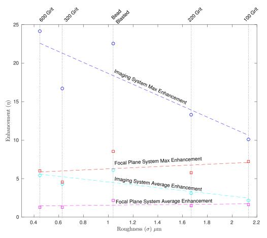
**Figure 3.** Enhancement ( $\eta$ ) vs. Surface Roughness ( $\sigma$ ). The surface roughness measured by the Tencor profilometer is plotted with enhancement. Linear trend lines are included. For the focal-plane system, maximum enhancement is shown in red, while average enhancement is shown in magenta. For the imaging system, maximum enhancement is shown in blue, while average enhancement is shown in cyan.
