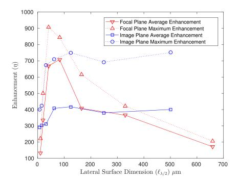
**Figure 5.** Simulated Enhancement ( $\eta$ ) vs. Lateral Surface Dimension ( $\ell_{\lambda/2}$ ). The red solid line shows average enhancement of the focal-plane system, while the red dotted line shows maximum enhancement. The solid blue line shows average enhancement of the imaging system, while the blue dotted line represents maximum enhancement.
