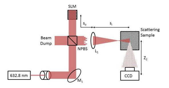
**Figure 2.** Image plane optical setup for reflective inverse diffusion. A vertically polarized HeNe laser is expanded, collimated, and normally incident on the SLM. The lens ( $L_1$ ) produces a demagnified image of the phase modulated beam onto the rough-surface reflector and the reflected speckle pattern is recorded by the CCD. The mirror ( $M_1$ ) and the NPBS are used to allow normal incidence with the SLM. The demagnification of the system is  $\frac{s_i}{s_0} \approx \frac{1}{8}$ .
