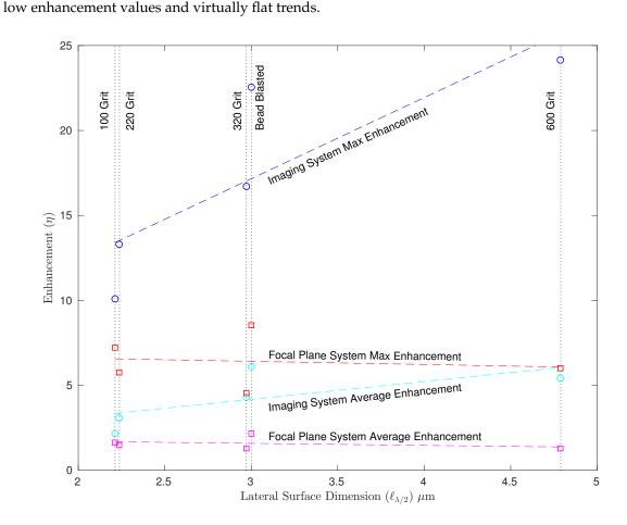
**Figure 4.** Enhancement ( $\eta$ ) vs. Lateral surface dimension ( $\ell_{\lambda/2}$ ). The lateral surface dimension,  $\ell_{\lambda/2}$ , is plotted with enhancement. The focal-plane system shows no change in enhancement with  $\ell_{\lambda/2}$ . However, the average enhancement of 1 indicates that the target segment has the same intensity as the background.
