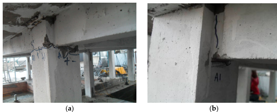
Figure 6. Model damage after Run 3. (a) Concrete crushing at the column end; (b) Slight crack at the beam end.
