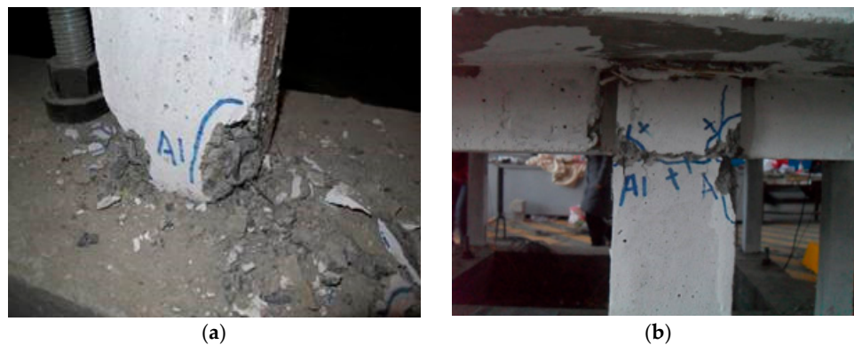
Figure 7. Model damage after Run 6. (a) Reinforcement buckling at the column root; (b) Concrete spalled at the column end.
