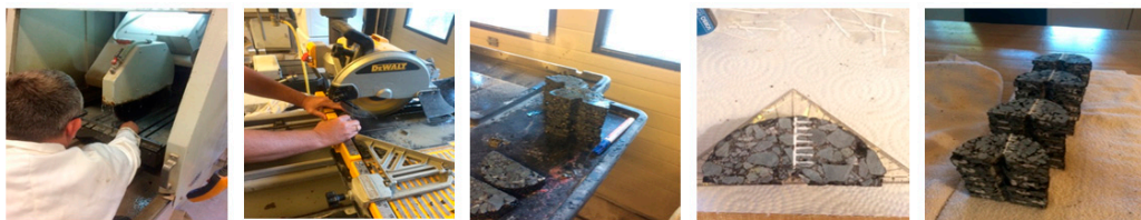
Figure 2. SCB test specimen cutting and marking process.
