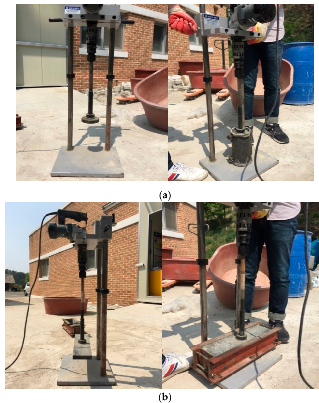
Figure 2. Manufacturing of test specimens. (a) Manufacturing of compressive strength specimens; (b) Manufacturing of flexural strength specimens.
