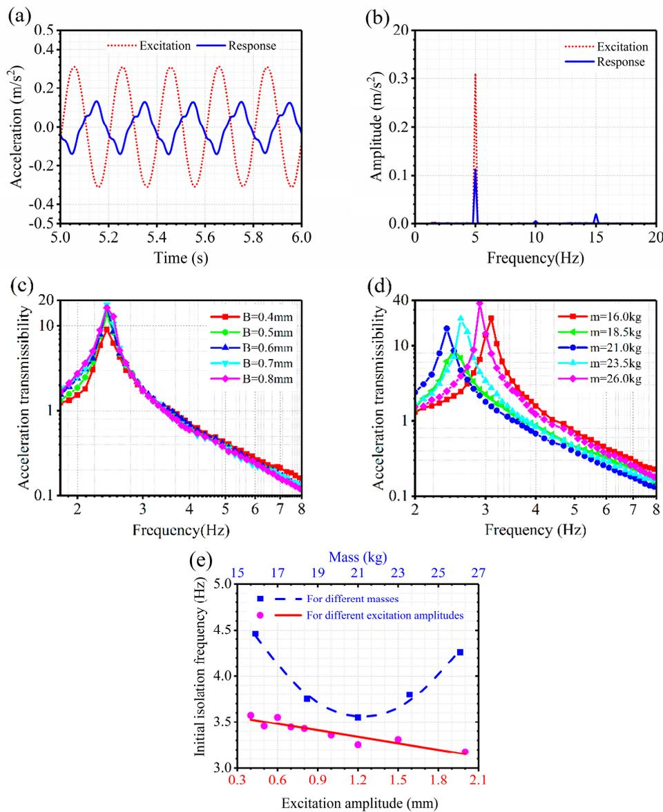
**Figure 9.** The results of discrete sinusoidal excitation experiment. (a) The time domain signal at 5 Hz with excitation displacement of 0.6 mm. (b) The frequency domain signal at 5 Hz with excitation displacement of 0.6 mm. (c) Acceleration transmissibility for different excitation amplitudes:  $m = 21$  kg. (d) Acceleration transmissibility for different mass loads with excitation amplitude of 0.6 mm. (e) The initial isolation frequency of the isolator.
