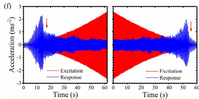
**Figure 10.** Time history signals of acceleration under linear sinusoidal sweep excitation. (a) Excitation displacement amplitude:  $B = 0.5$  mm. (b)  $B = 1.0$  mm. (c)  $B = 1.5$  mm. (d)  $B = 1.5$  mm. (e)  $B = 2.5$  mm. (f)  $B = 3.0$  mm.
