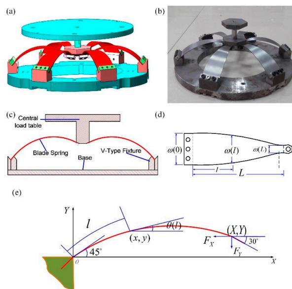
**Figure 1.** The model of the geometric anti-spring isolator. (a) Schematic of the geometric anti-spring isolator. (b) Photograph of the geometric anti-spring isolator. (c) Cross-section diagrams of the geometric anti-spring isolator. (d) The shape of the cantilever blade spring. (e) One dimension mechanical model of the blade spring.
