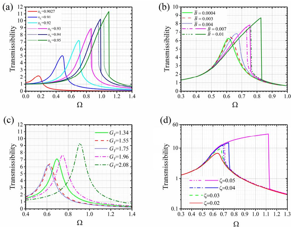
**Figure 6.** The mathematical simulation results. (a) Transmissibility for different nonlinear geometric parameters at the rated load. (b) Transmissibility for different excitation displacement amplitudes. (c) Transmissibility for different load weights. (d) Transmissibility for different damping ratios.
