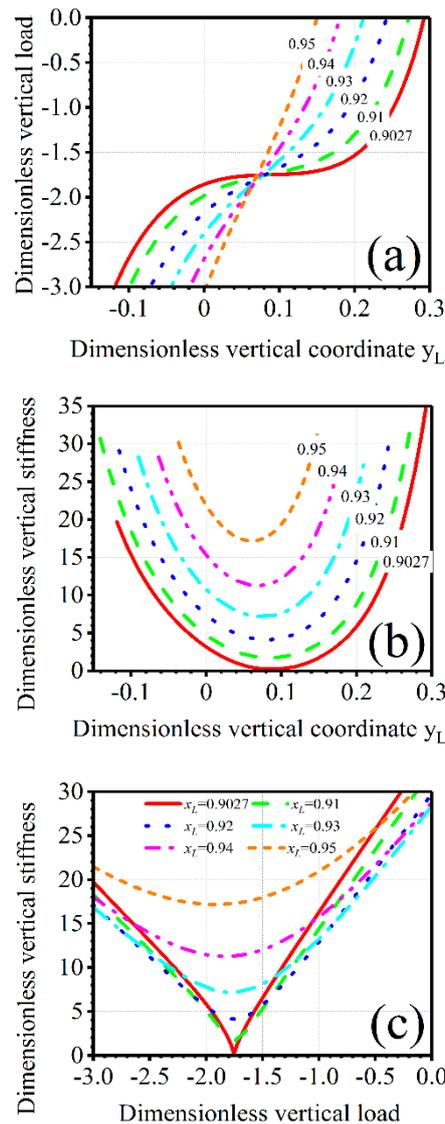
**Figure 3.** Dimensionless theoretically numerical result of the geometric anti-spring isolator. (a) Dimensionless vertical force. (b) Dimensionless vertical stiffness vs. vertical coordinate. (c) Dimensionless vertical stiffness vs. vertical force.
