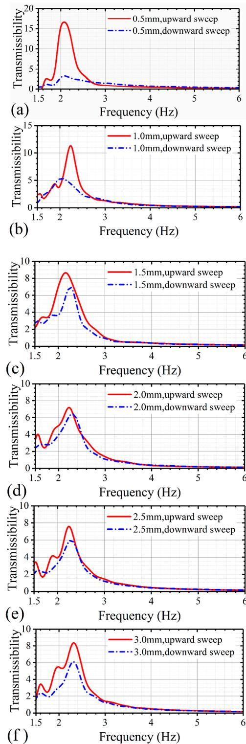
**Figure 11.** Acceleration transmissibility of the geometric anti-spring isolator under linear frequency sweep excitation with different excitation displacement amplitudes. The excitation displacement are: (a) 0.5 mm, (b) 1.0 mm, (c) 1.5 mm, (d) 2.0 mm, (e) 2.5 mm and (f) 3.0 mm, respectively.
