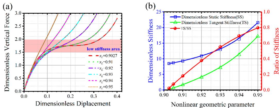
**Figure 4.** Dimensionless vertical force (a) and stiffness characteristic at the optimal working point (b) of the geometric anti-spring isolator.
