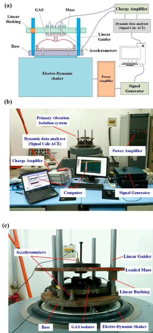
**Figure 8.** Dynamic experimental system for the geometric anti-spring isolator. (a) Schematic of the dynamic experimental setup; (b) Photograph of the dynamic experimental setup; (c) Photograph of the primary vibration isolation system.
