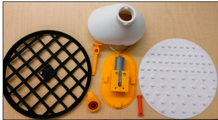
Figure 1. Disassembled 3-D printed components of the open source nutating mixer.
