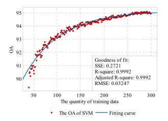
Figure 18. The exponential curve fit to the performance results of the SVM.
