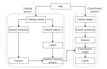
Figure 1. Flow chart illustration of classification modeling.
