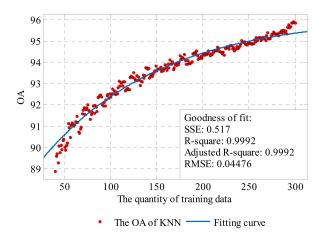
Figure 17. The exponential curve fit to the performance results of the KNN.
