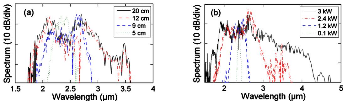
**Figure 11.** Evolution of experimental SC spectra recorded at the output of the tellurite step-index fiber with a core diameter of  $3.5\ \mu\text{m}$  (i.e., with two ZDWs) when pump wavelength is fixed to  $2300\ \text{nm}$ . (a) Evolution as a function of fiber length for an input peak power of  $2.2\ \text{kW}$ . (b) Evolution as a function of input peak power for a fiber length of  $12\ \text{cm}$ .
