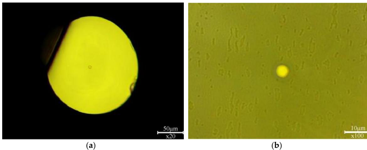
**Figure 3.** Cross-section of the small core step-index fibre under optical binocular with (a) a  $\times 20$  objective and (b) a  $\times 100$  objective.
