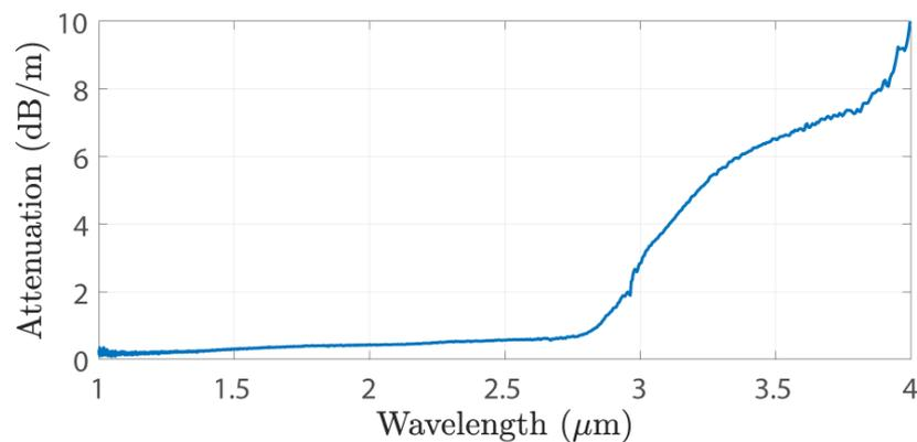
**Figure 2.** Large-core (TZNF/TZNG) fiber losses measured by means of the cutback method.
