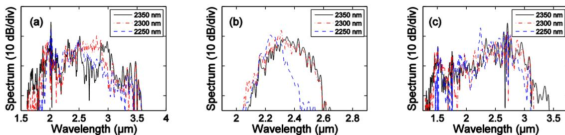
**Figure 12.** Evolution of experimental SC spectra recorded as a function of pump wavelength for a fixed input peak power of  $\sim 2.5\ \text{kW}$  for  $12\text{-cm}$ -long segments of tellurite step-index fiber with a distinct core diameter, namely (a)  $3.5\ \mu\text{m}$ , (b)  $3\ \mu\text{m}$ , and (c)  $4\ \mu\text{m}$ .
