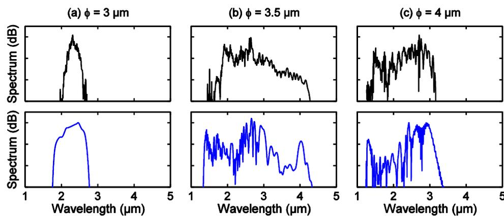
**Figure 13.** (Top panels) Optimized SC spectra recorded with 12-cm-long segments of tellurite step-index fiber with a distinct core diameter, namely (a) 3  $\mu\text{m}$ , (b) 3.5  $\mu\text{m}$ , and (c) 4  $\mu\text{m}$ . The pump wavelength was fixed to 2300 nm and the input peak power is  $\sim 3$  kW. (Bottom panels) Corresponding numerical simulations are shown with dashed blue lines.
