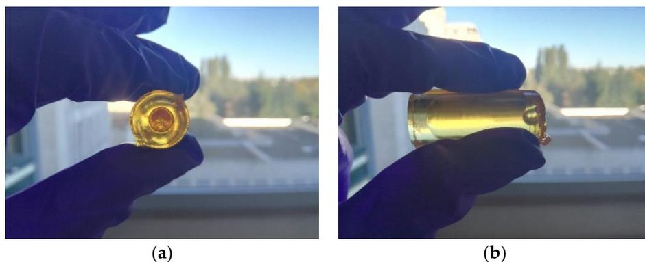
**Figure 1.** Pictures of the cross-section (a) and side-section (b) of the step-index preform synthesized with the built-in-casting method.
