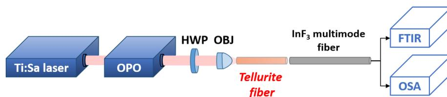
**Figure 10.** Experimental set-up used for mid-IR supercontinuum generation. OPO: optical parametric oscillator. HWP: half-wave plate. OBJ: 20 × microscope objective lens. FTIR: Fourier-transform infrared spectrometer. OSA: optical spectrum analyzer.
