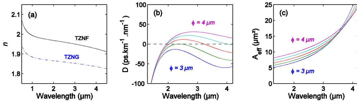
**Figure 4.** (a) Refractive index curves of both TZNF core and TZNG cladding glasses. (b) and (c) Wavelength-dependent curves of dispersion parameter  $D$  and effective mode area  $A_{\text{eff}}$  of the fundamental guided mode in distinct step-index tellurite fibers with respective core diameters  $\phi = 3, 3.25, 3.5, 3.75,$  and  $4 \mu\text{m}$ .
