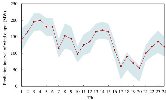
Figure 2. Prediction interval of wind output though a day.
