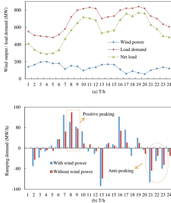
**Figure 1.** Load demand/wind output under four seasons; (a) net load fluctuation with and without wind power integration; and, (b) ramping demand of systems with and without wind power.
