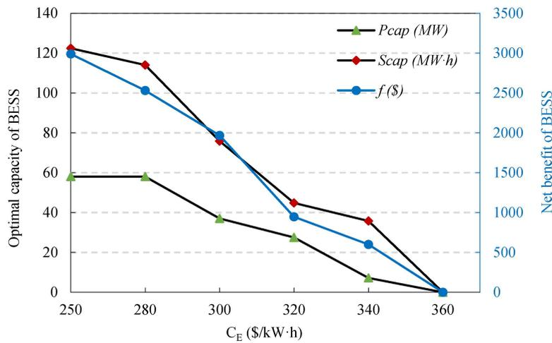
Figure 8. Optimal results under different investment costs of BESS.  $C_E$ : unit capacity cost of BESS.
