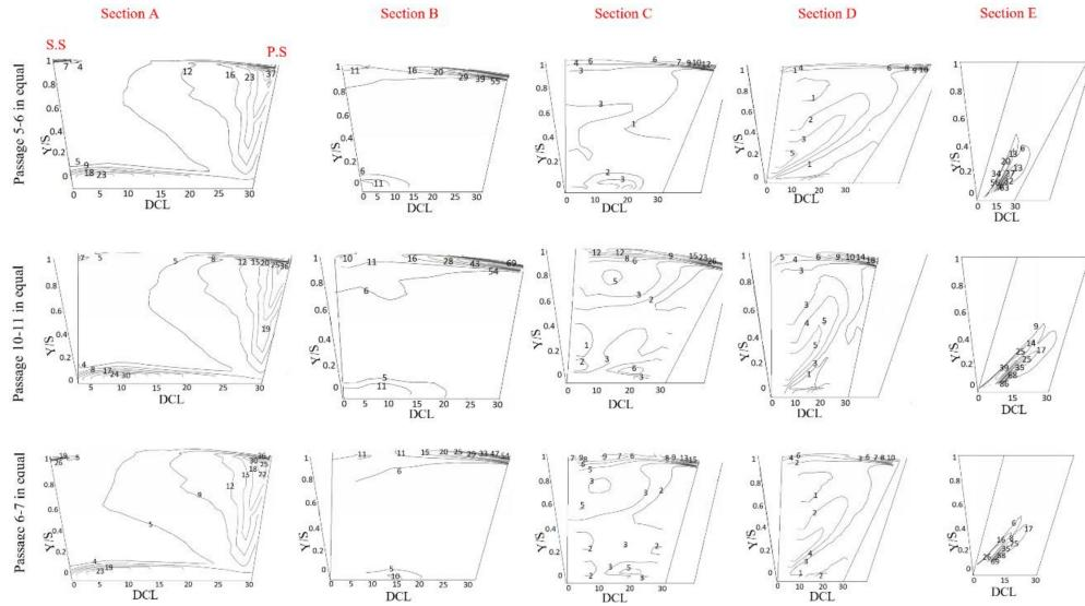
**Figure 8.** Vorticity contours at specified sections in blade passages 5–6, 10–11, and 6–7 of the equal case in spanwise location against the degree in circumferential location (DCL).
