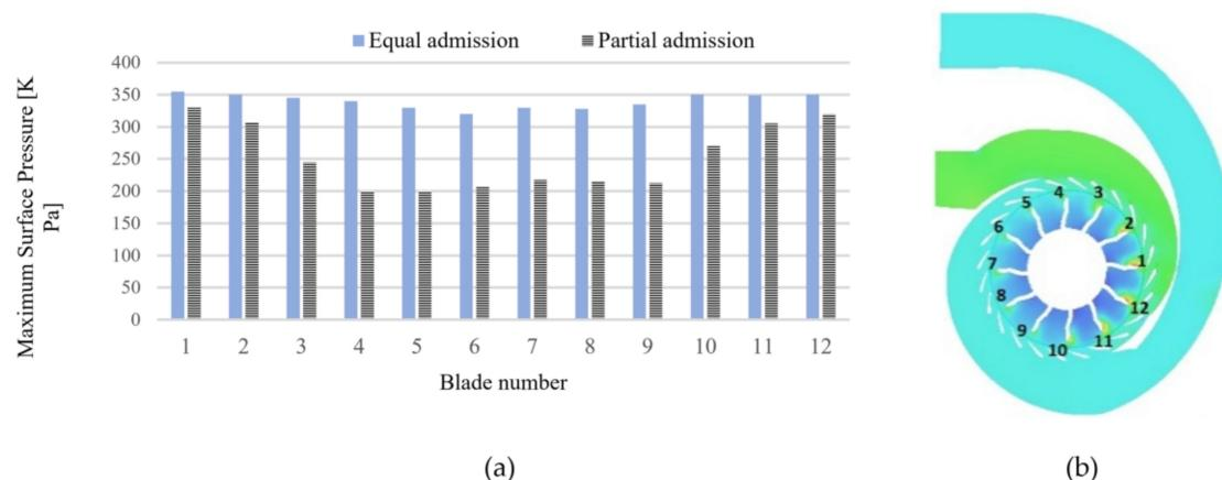
**Figure 5.** (a) Surface pressure on the all of the turbine blades in equal and partial admission; (b) definition of blade passages.
