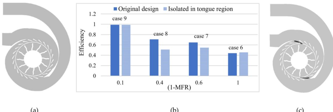
**Figure 7.** (a) Original geometry; (b) efficiency drop with increasing the pressure inequality of two limbs (c) separated in tongue region (A and B).
