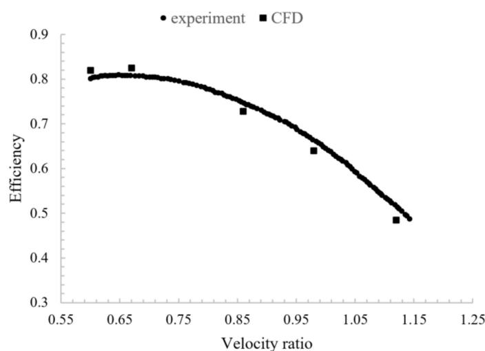
**Figure 3.** Comparison of computed and measured efficiency against velocity ratio.
