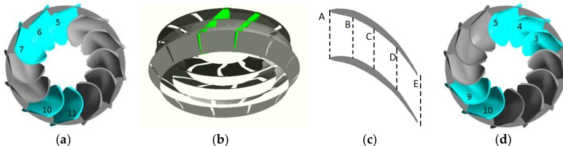
**Figure 6.** Selected passages and sections on the turbine blades (a) in equal admission; (b) in three-dimensional (3D) view; (c) in two-dimensional (2D) view; (d) in partial admission.
