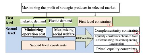
Figure 2. The conversion of the bi-level optimization solution to a single-level.
