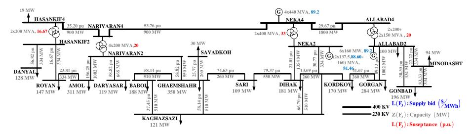
Figure 9. Single-line diagram of the MAZANDARAN Regional Electric Company (MREC) transmission network.
